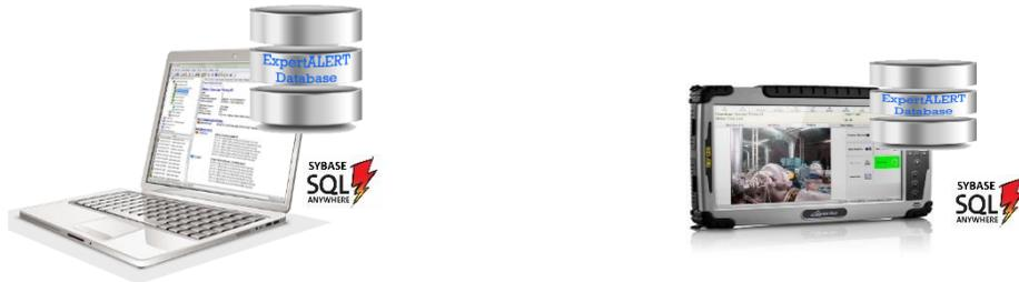
The advantage of a local installation is the simplicity of the setup. A local system contains the ALERT software, the ALERT database, and the Sybase engine. However, this setup also has the highest risk given backups are generally manual and often forgotten. Also, unless working only directly from the TRIO Data Collector, this setup is the most complicated for communication between two or more users.
