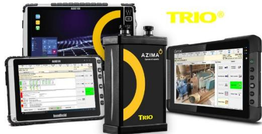
Capacitive touchscreens are brighter given there are fewer layers needed for input. The input has less interference from debris, scratches or small cracks than resistive touchscreens. They are also not subjective to dead spots from frequent, repeated use or the need to re-calibrate.
